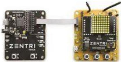
The ADK-W01 is a starter kit for developing secure Wi-Fi networking applications with ZentriOS and the ZentriOS SDK.
