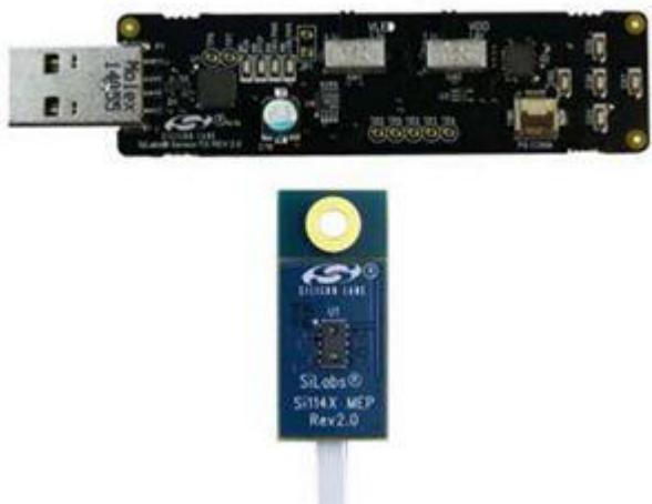
The Si1143 Module Evaluation Kit and accompanying Si114x Programmer's Toolkit software allow quick and easy access to the features and functions of the Si1143-M01, Si1142-M01, and Si1141-M01 optical sensors while enabling the evaluation of the sensor's performance.
