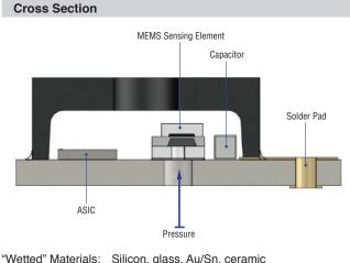
Silicon, glass, Au/Sn, ceramic (Ported version also contains Au and solder) Any material in contact with the media is considered a "wetted" material.
