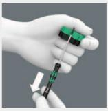
To demagnetise the tool, simply run it down one of the four negative sides. See page 58.
