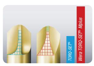
Wera developed the Mplus profile with stronger flanks compared with tools with a conventional TORQ-SET® profile. This results in approximately 70 % extra torsional strength and greatly extends the service life of Wera Mplus tools.
