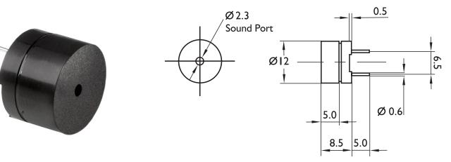
**Dimensions : Millimetres** Tolerance: ±0.5mm
