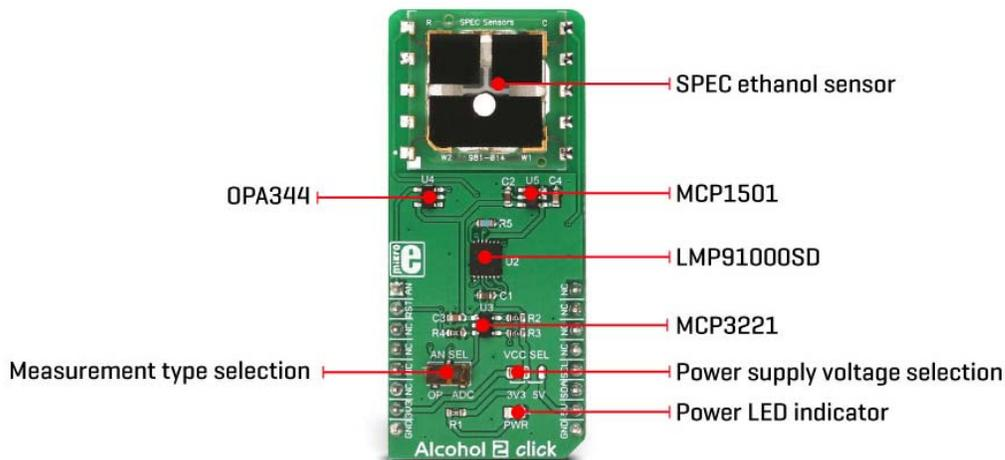
Although very reliable and accurate, this sensor is great for building relative gas sensing applications. For example, it can detect increased levels of ethanol gas. However, when developing applications for the absolute gas concentration, the sensor needs to be calibrated and the measurement data needs to be compensated.
