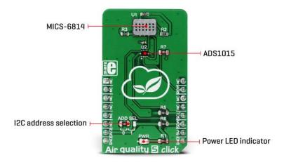
As mentioned, there are three sensors on the same die. Each of them reacts with a different type of gas. There is a RED sensor which reacts with the reducing gas agents, an OX sensor which reacts with the oxidizing gas agents, and lastly, a sensor which reacts with NH3. These sensors provide readings (in ppm) for eight different gasses, which are of interest to be monitored in the automotive, industry or agriculture polluted atmosphere.
