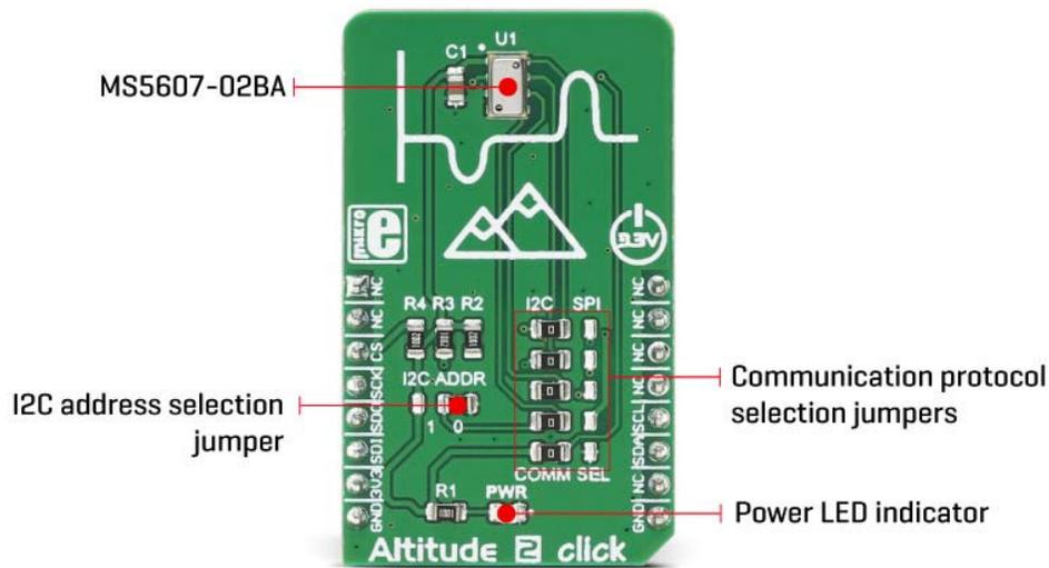
Each sensor IC is factory calibrated at two temperatures and pressures. The calibration coefficients are stored to its 128 bit PROM area. To calculate the correct values, these coefficients need to be used in the calculation, in order to derive real values from the
