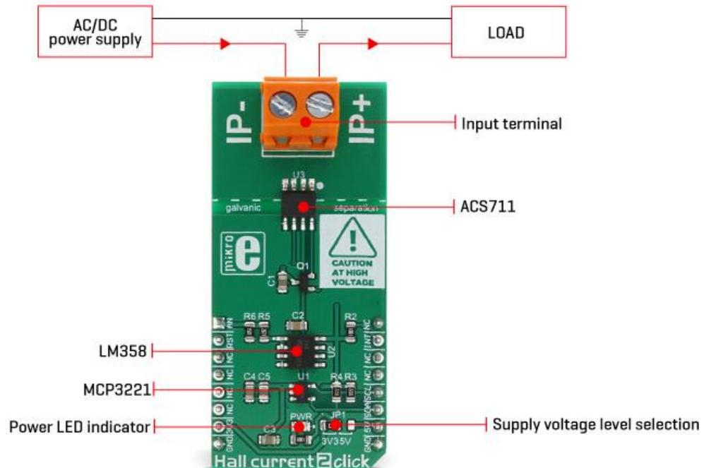
The output voltage changes linearly with the input current, in steps of 110mV/A. To allow conversion via the external ADC, the output voltage is passed through the buffering circuit, comprised of the LM358 - a low noise operational amplifier in a unity gain configuration.
