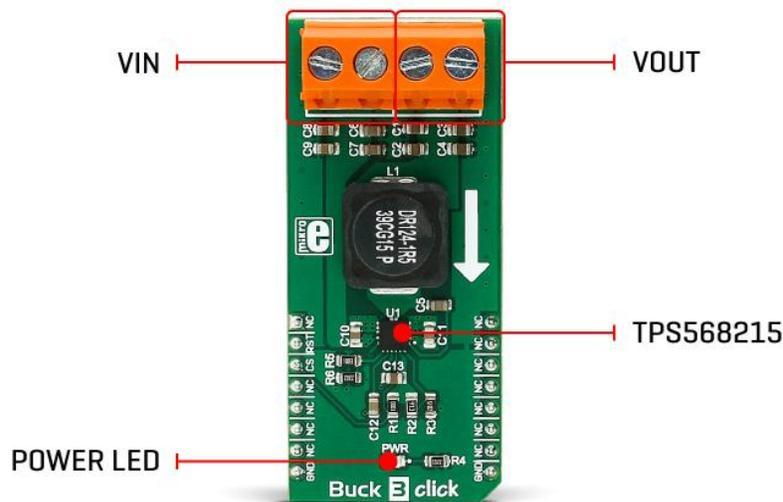
The onboard voltage divider connected to the MODE pin of the IC is used to set the device to work with the fixed PWM frequency of 800kHz, DCM/Eco-mode™ for light loads, and to set the limiting current to about 7A.
