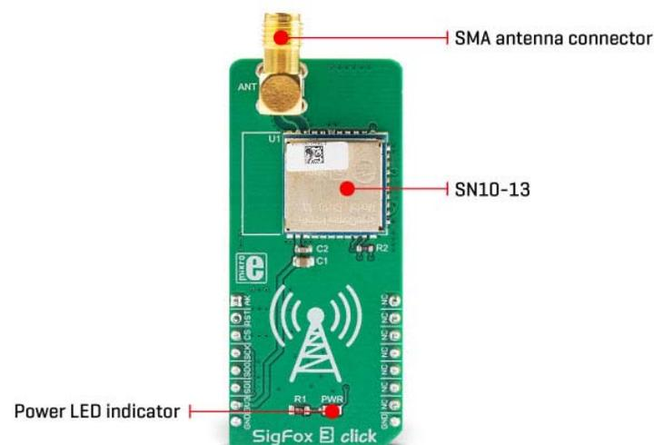
The Click board™ is equipped with the SN10-13 Sigfox™ certified module, manufactured by InnoComm Mobile Technology Corporation. The heart of this module is the NXP 0L2385, a sub-GHz wireless transceiver System-on-Chip (SoC). The communication
