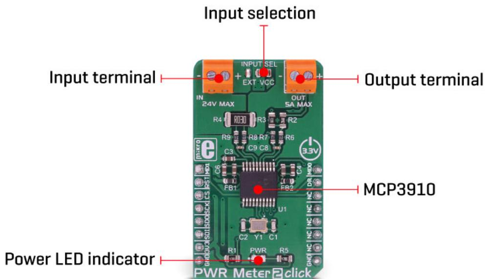
The Click board™ is clocked by a 20MHz crystal. However, it is up to the user to set the pre-scalers correctly, according to the datasheet of the MCP3910. However, the included library offers functions which take care about correct settings. High clock speed allows maximum oversampling rate (OSR) to be used, allowing the best performance to be achieved, but consuming more power at the same time.
