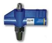
HS Static Control Nozzles are "shockless" nozzles. The term shockless indicates that the ionizing point, located inside the nozzle tip, is capacitively coupled to the high voltage source, thus limiting the current at the point to a very low level. Under normal conditions, direct contact with the point will not result in a shock sensation. HS Static Control Nozzles can be installed individually, in series, and mounted on a standard air bar header.
