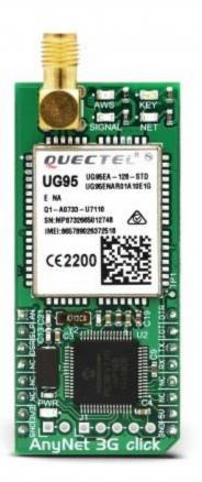
**AnyNet 3G-EA click** is a cellular to AWS gateway device, which provides developers with the complete solution for various IoT applications, by using the AWS IoT and Cloud Storage services for the data storage, analyzing and
