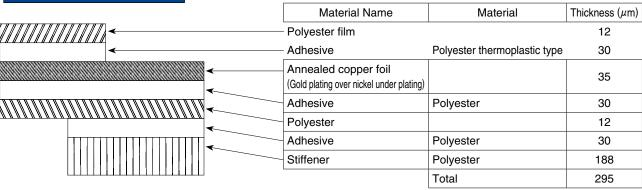
\* Actual tolerance of the thickness is approximately  $\pm 20 \mu m$ .
