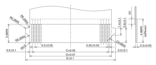
Note 1 : Stiffener dimension should be 3.5mm min., and X dimension should be 0.5mm for improved flexibility of FPC.
