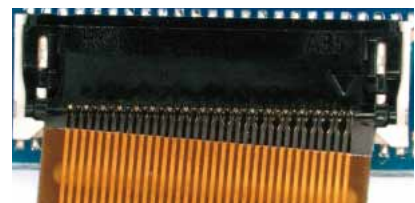
FPC is inserted diagonally.
