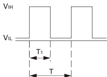
$$V_{IH}=4.75 \text{ V to } 5.25 \text{ V}$$
