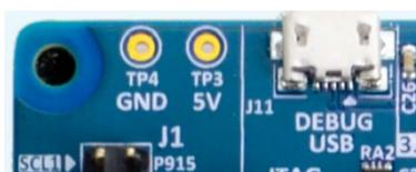
Figure 4 USB debug connector (J11), TP3, and TP4 on target board
