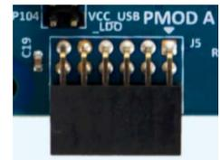
Please note that signals on PMOD A are shared with Main MCU pin header J1 and J2. Care must be taken to ensure shared signals are not used concurrently.
