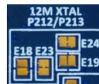
The MCU pins for the 12 MHz clock crystal may be connected to P212 and P213. To disconnect the 12 MHz crystal, open copper jumpers E23 and E24, and close copper jumpers E18 and E19.
