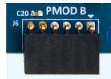
Note that signals on PMOD B are shared with Main MCU pin header J1 & J2. Care must be taken to ensure shared signals are not used concurrently.
