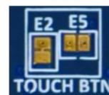
To disconnect the Capacitive Touch Button from the MCU, copper jumper E2 must be open.
