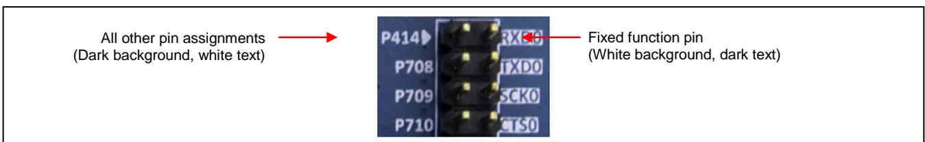
Figure 20 Fixed function pin label example
