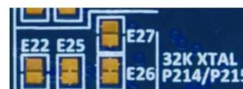
The MCU pins for the 32.768 kHz clock crystal may be connected to P214 and P215. To disconnect the 32.768 kHz crystal, open copper jumpers E25 and E26, and close copper jumpers E22 and E27.
