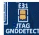
The J-Link OB interface is multiplexed with the JTAG interface, and can collectively be referred to as the Programming Interface. While the J-Link OB interface and the JTAG interface do not conflict, the J-Link OB signals may be isolated from the programming interface by changing the copper jumpers as described in Section 4.4.2, Debug USB.
