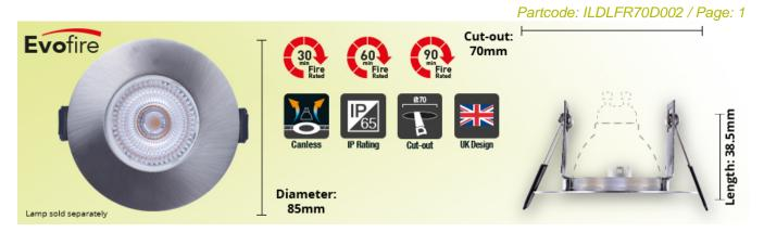
The Evofire Fire Rated Downlight is a safe and attractive fitting for a GU10 LED lamp. The fully open design of the Evofire does not conceal your lamp in a large metal canister, which can trap some of the heat it generates, lowering lamp lifetime and performance. Lamps installed in an Evofire run at up to 10 degrees C cooler than a typical can-style fire rated downlight from leading LED brands - this can extend the lifetime of your lamps.
