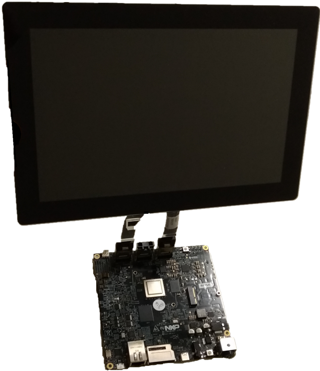
Figure 10. Dual-channel LVDS panel example
