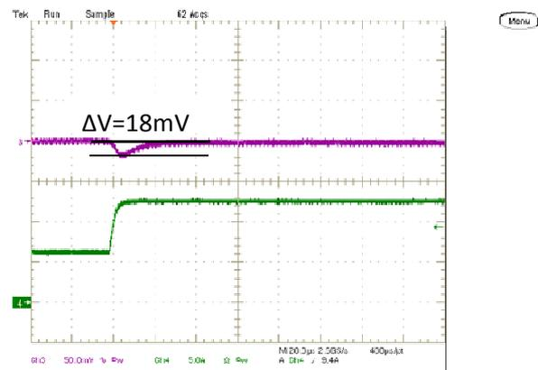
Step Load Transient Response (Vin=5.0V, Vout=0.7V, Load=660uF,
