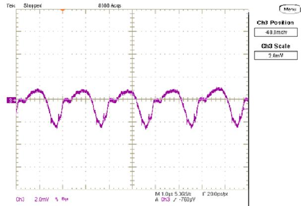
Step Load Transient Response (Vin=12.0V, Vout=1.8V, Cload=660uF,
