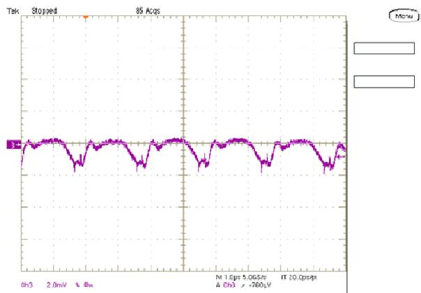
Step Load Transient Response (Vin=12.0V, Vout=1.0V, Cload=660uF,
