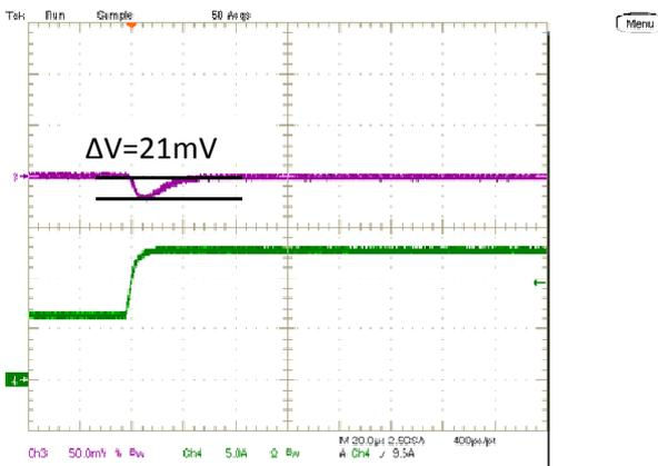
Step Load Transient Response (Vin=12.0V, Vout=0.7V, Cload=660uF,
