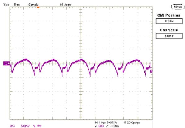
Step Load Transient Response (Vin=5.0V, Vout=1.8V, Load=660uF,
