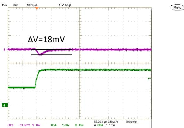
Step Load Transient Response (Vin=5.0V, Vout=1.0V, Load=660uF,
