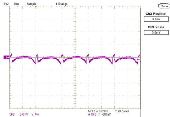
Step Load Transient Response (Vin=5.0V, Vout=1.0V, Load=660uF,
