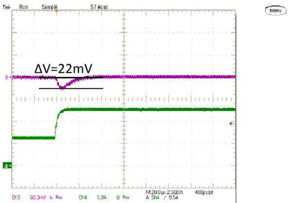
Step Load Transient Response (Vin=12.0V, Vout=1.8V, Cload=660uF,
