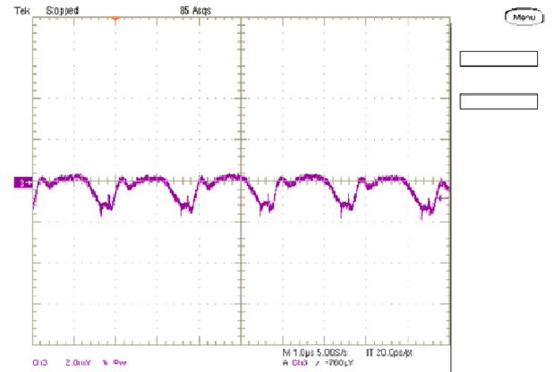
Step Load Transient Response (Vin=12.0V, Vout=0.7V, Cload=660uF,
