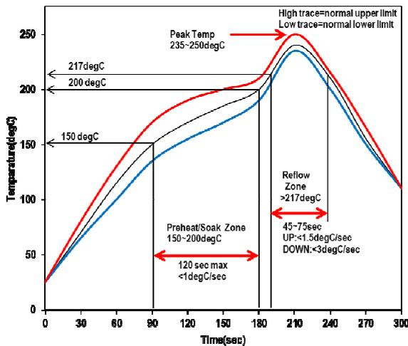
**CAUTION: Do not reflow the converter as follows, because the converter may fall from the substrate during reflowing.**
