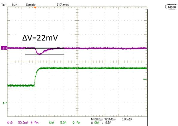
Step Load Transient Response (Vin=12.0V, Vout=1.0V, Cload=660uF,
