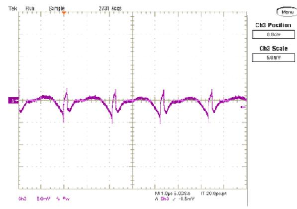
Step Load Transient Response (Vin=5.0V, Vout=0.7V, Load=660uF,
