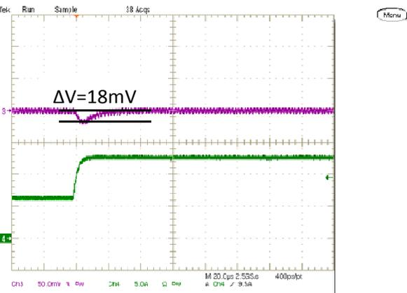
Step Load Transient Response (Vin=5.0V, Vout=1.8V, Load=660uF,
