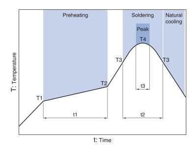
Preheating Soldering Peak Time Temp. Time Time Temp. Temp. T2 t3 180°C 60 to 120s 10 to 30s 245°C 150°C 230°C 5s
