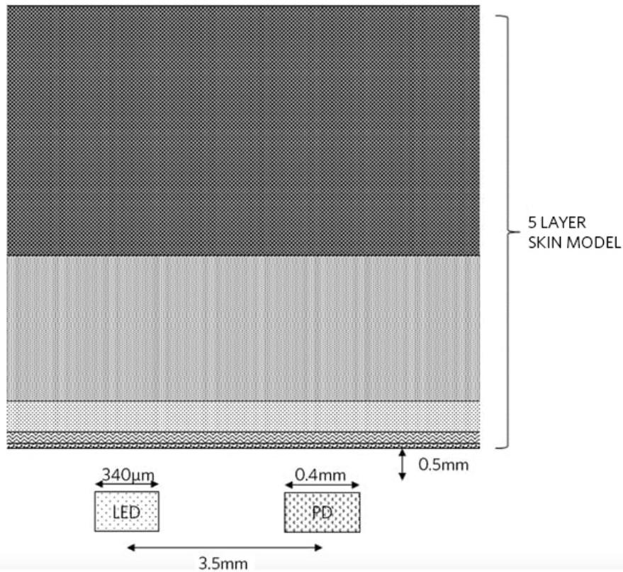
Figure 3. Dimensions of biosensor configuration used in simulation.
