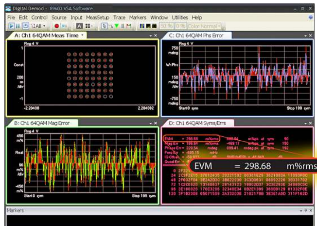
Figure 3. Constellation diagram and EVM of a 64-QAM baseband signal
