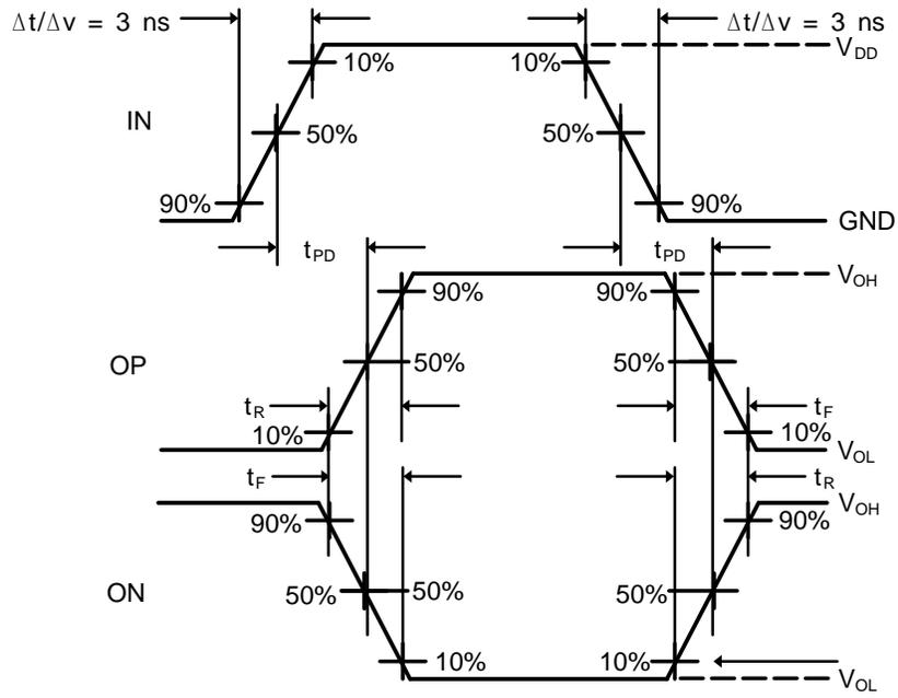
Figure 2. Switching Waveforms
