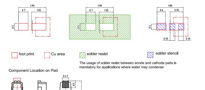
For superior solder joint connectivity results we recommend soldering under standard nitrogen atmosphere.
