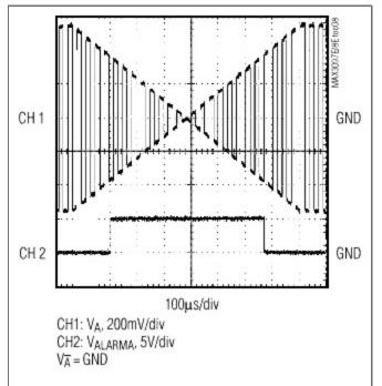
Figure 8. Detecting poor signal strength.
