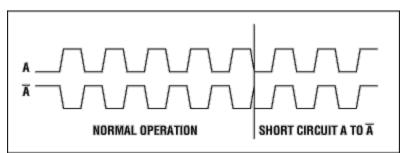
Figure 7. Detecting shorts between differential signals.
