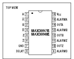
Figure 4. MAX3097 pinout.
