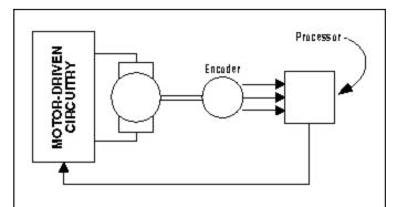
Figure 1. The major building blocks of processor-controlled electric motors.
