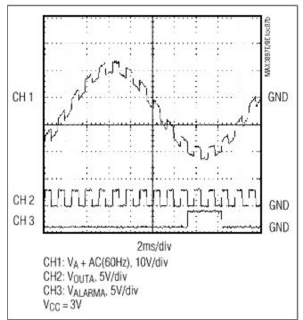
Figure 5. This shows the fault alarm on channel A due to the excessive common-mode range; the fault
