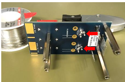
Step 4 TO-220 sockets soldering
