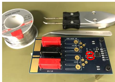
Step 5 MOSFETs placement into the sockets
