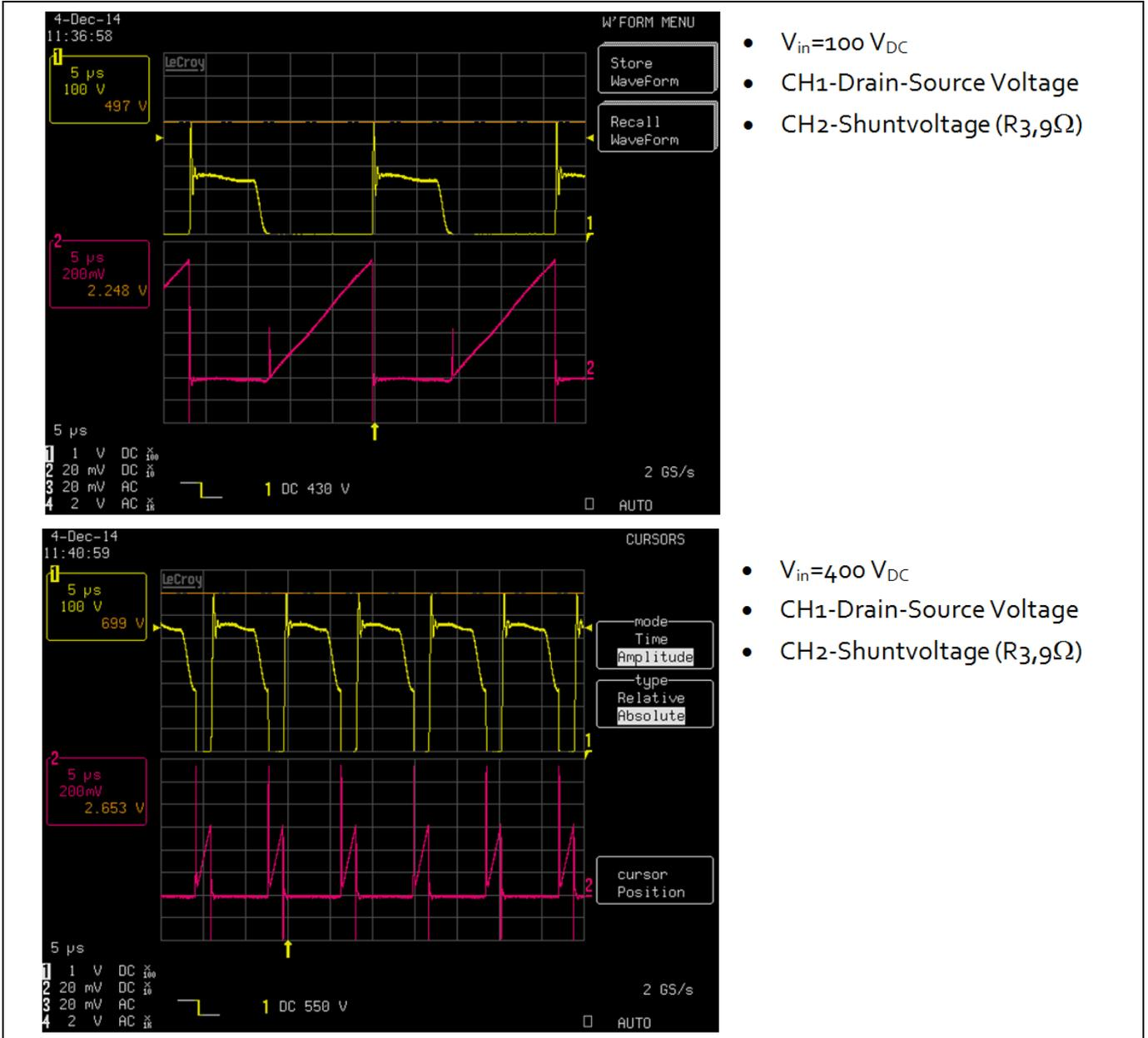
Figure 12 Waveforms of the auxiliary power supply
