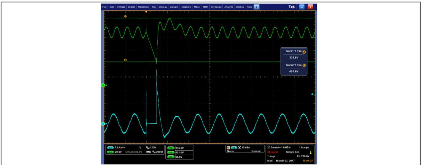
Figure 24 AC line drop out for 10 ms when  $V_{IN} = 230 \text{ V AC}$  at  $P_{OUT} = 800 \text{ W}$
