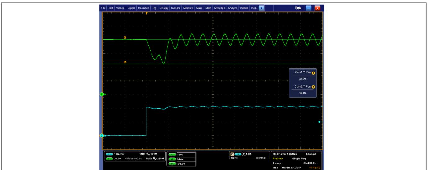
Figure 19 Load step: 0% → 100% at  $V_{IN} = 230$  V AC
