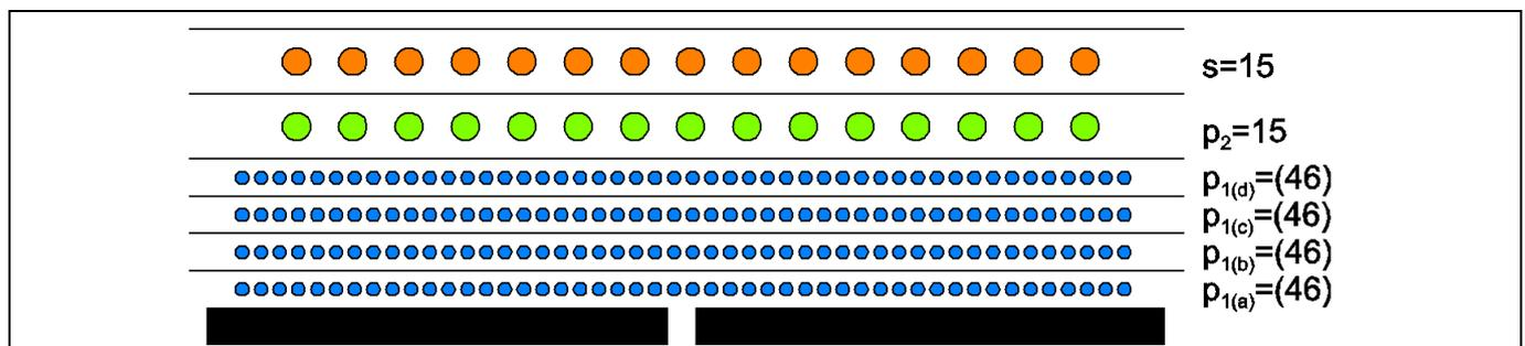
Figure 10 Winding arrangement
