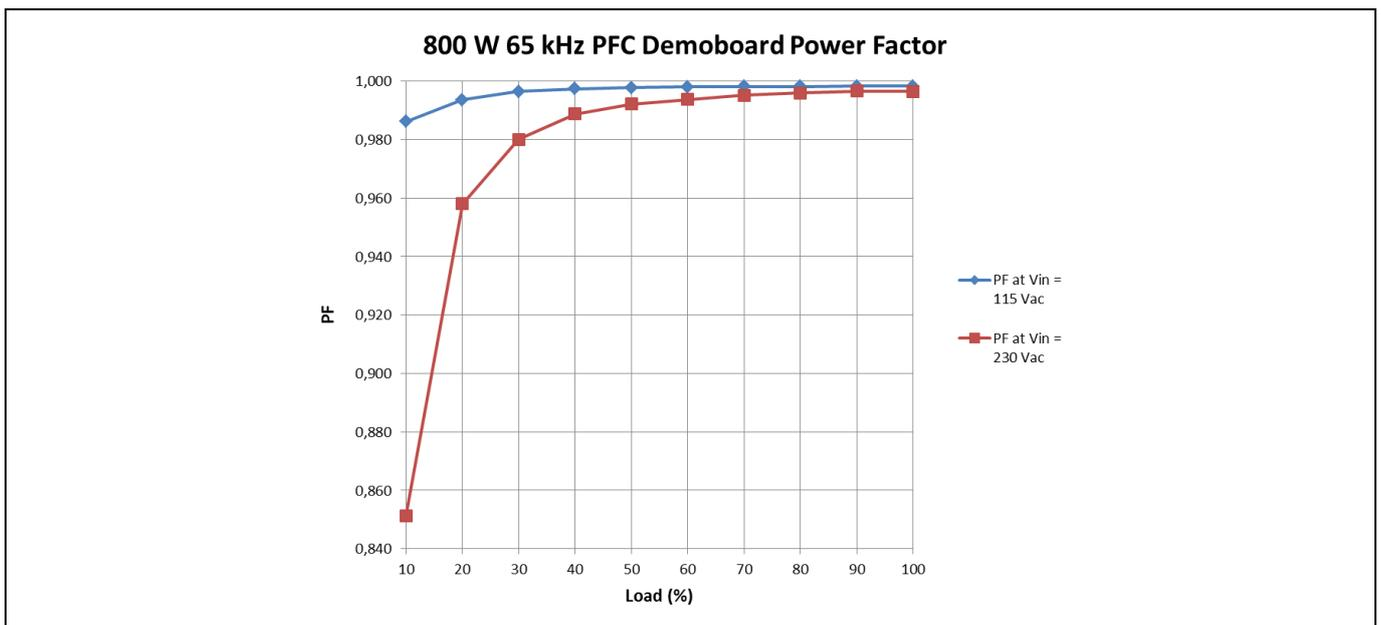
Figure 14 Power factor at high and low line
