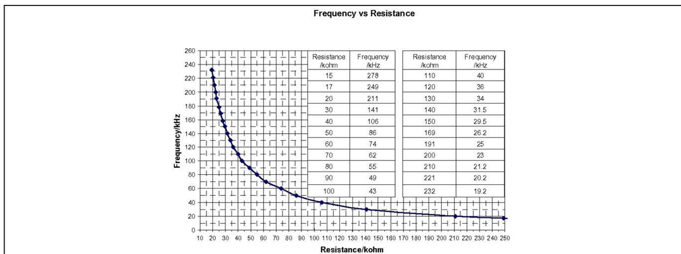
Figure 9 Frequency setting in the ICE3PCS01G IC
