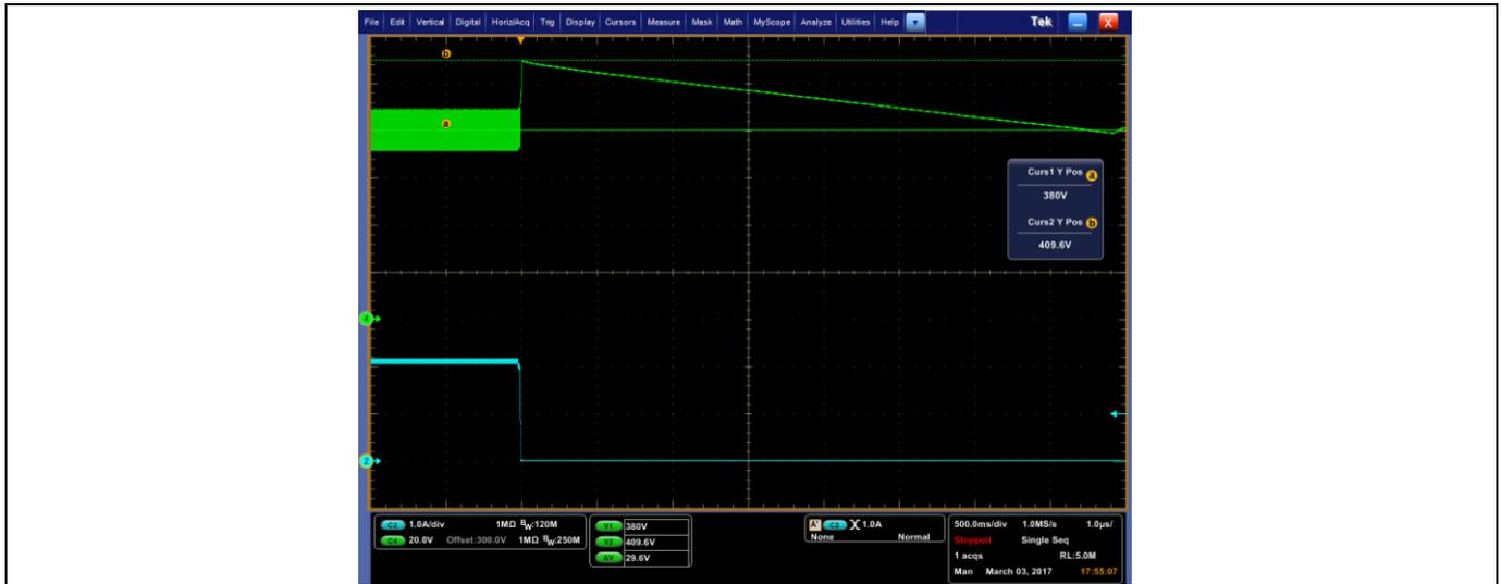
Figure 20 Load step: 100% → 0% at  $V_{IN} = 115$  V AC
