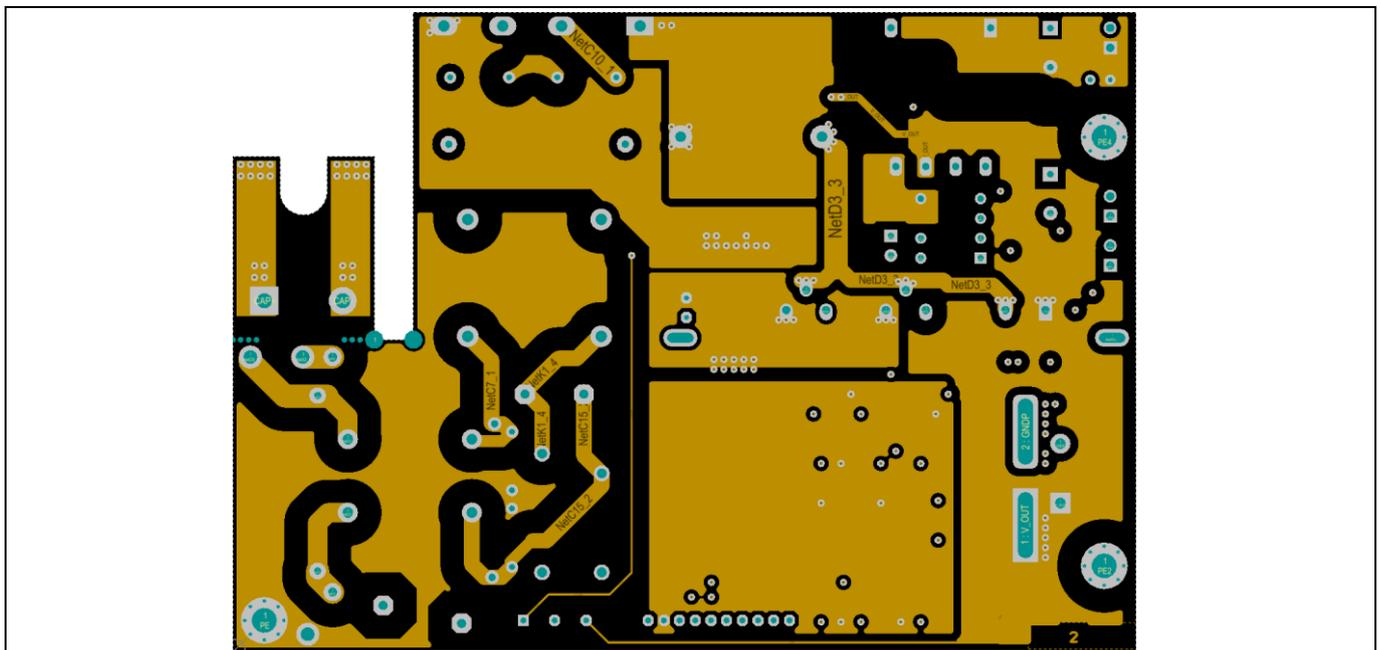
Figure 30 View of PCB inner 1 layer
