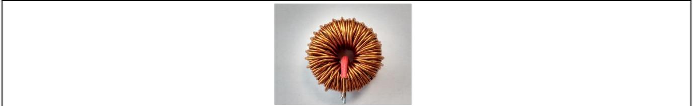
Figure 5 Picture of the PFC choke
