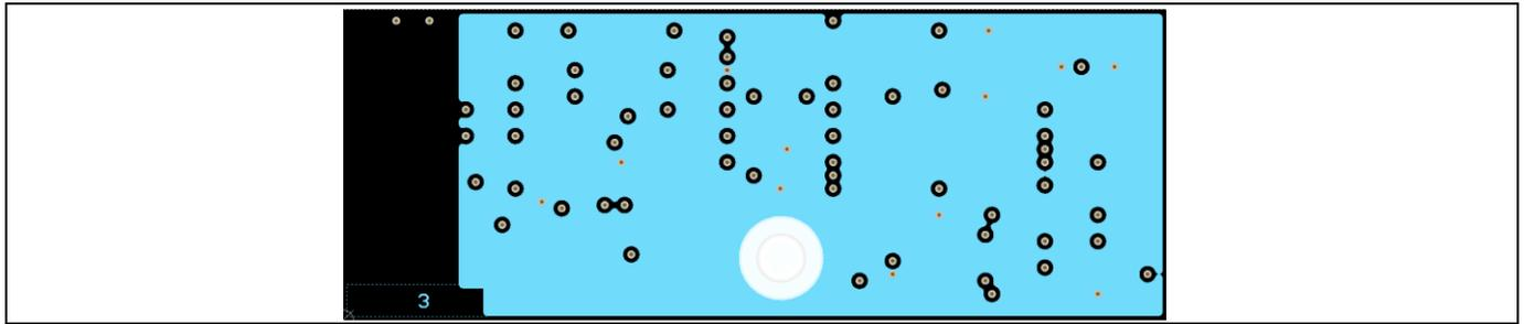
Figure 38 View of analog control PCB inner 2 layer
