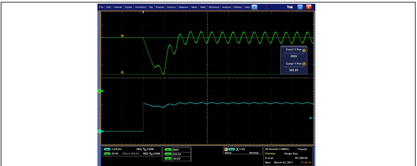
Figure 18 Load step: 0% → 100% at  $V_{IN} = 115$  V AC
