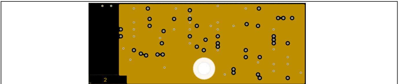
Figure 37 View of analog control PCB inner 1 layer
