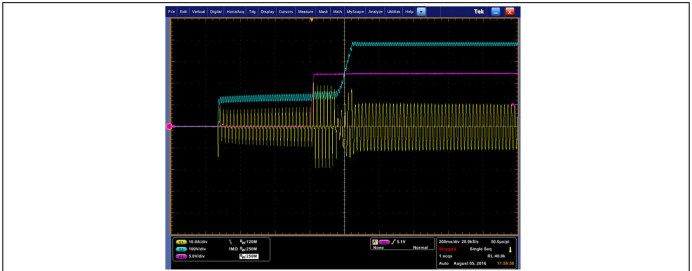
Figure 21 Star-up at  $V_{IN} = 115$  V DC
