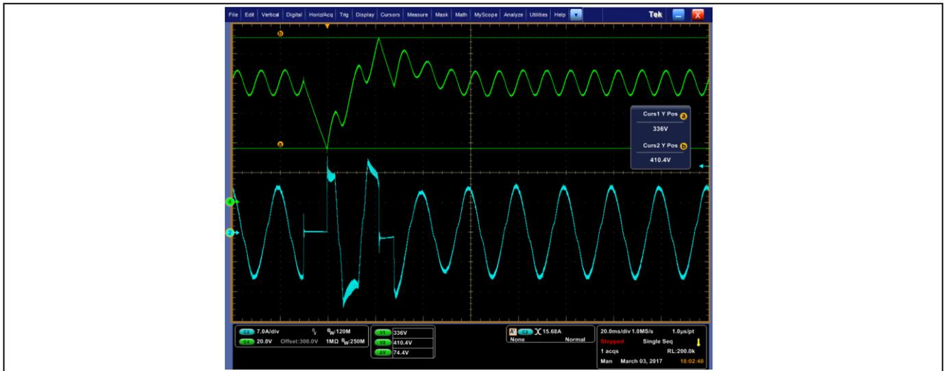
Figure 23 AC line drop out for 10 ms when  $V_{IN} = 115$  V AC at  $P_{OUT} = 800$  W
