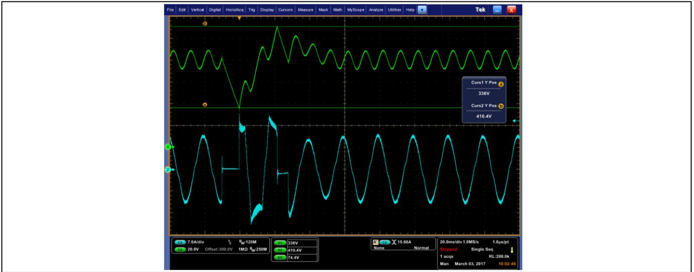
Figure 23 AC line drop out for 10 ms when  $V_{IN} = 115 \text{ V AC}$  at  $P_{OUT} = 800 \text{ W}$
