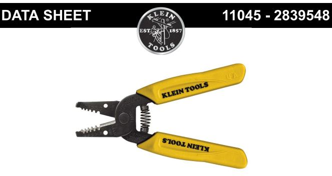
This compact, lightweight wire-stripping and cutting tool is designed to cut 10-18 AWG solid wire. The precision-ground stripping holes cut wire cleanly and aid in easy removal of insulation. A narrow nose helps this tool fit easily into tight places.
