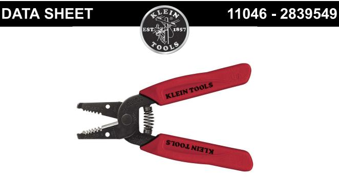
This Klein Tools Wire Stripper/Cutter cuts, strips, loops and gauges 16-26 AWG stranded wire. The precision-ground stripping holes cut wire cleanly and aid in easy removal of insulation. A narrow nose helps this tool fit easily into tight places.
