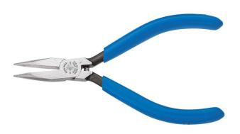
Lightweight, slim-nose pliers for precision subminiature assembly work. Polished inside jaws help prevent nicking of wire. Curved handles provide greater tool control. Spring-loaded for self-opening action. Hot-riveted joint for smooth action and no handle wobble.
