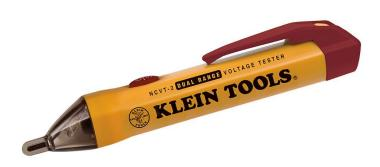
This Dual-Range Non-Contact Voltage Tester automatically detects low and standard voltage. A bright-green LED will tell you that the tester is working, and also functions as a work light. The red light flashes and two distinct warning tones sound when either low or standard voltage is detected.
