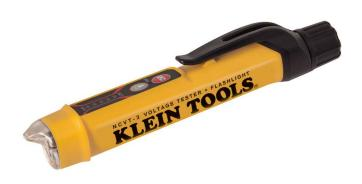
The NCVT-3 is a non-contact voltage tester with an integrated torch. The voltage sensor detects 12-1,000 V AC and indicates the presence of voltage in cables, cords, circuit breakers, light fixtures, switches, outlets and wires, as well as AC voltage in doorbells, thermostats, low-voltage lighting and irrigation systems. Includes both visual and audible signals. The NCVT-3 is rugged enough for any job site.
