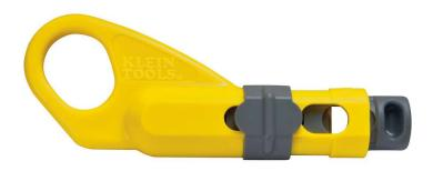
Klein Tools' Coax Combination Radial Stripper works on both standard and utility-sized cables. The durable, high-carbon steel cutting blades automatically adjust to different cable diameters. Klein's exclusive sliding depth gauge pre-measures cables for fast, accurate and repeatable stripping every time.
