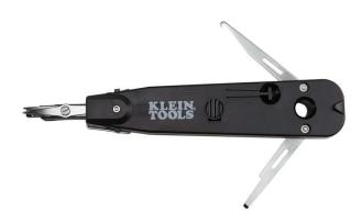
Specifically designed for use on Krone blocks and network infrastructure. Built-in swing-out combination hook and spudger conveniently helps manipulate wire and small components. A panel sensor detects the presence of a Krone punch-down panel, allowing the mechanism to seat and cut the wire. Lock the impact mechanism easily simply by rotating the impact lock dial.
