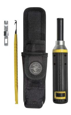
The Cushion-Grip Impact Tool Kit provides everything required to install and maintain 110 and 66 panels, cross-connect systems and wall jacks with secure terminations. Using an optimised two-step impact process, the punch-down tool inserts and then trims off excess wire precisely. The 4-piece kit comes with punch-down tool, wire extractor, blade and pouch.
