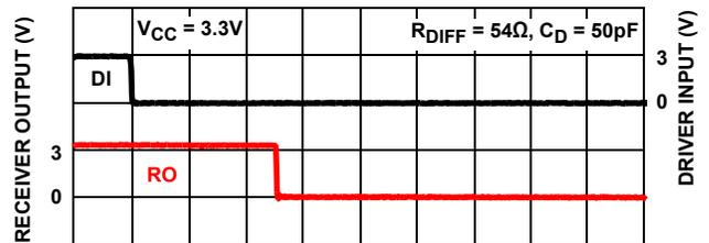
FIGURE 37. ISL32602E, ISL32603E DRIVER AND RECEIVER WAVEFORMS, HIGH TO LOW
