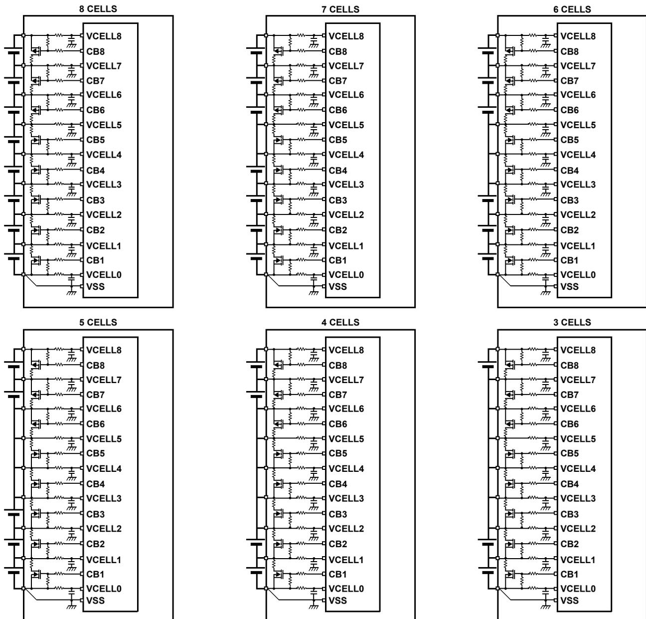
FIGURE 55. BATTERY CONNECTION OPTIONS USING THE ISL94203EVKIT1Z BOARD
