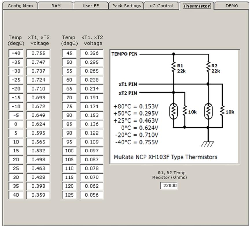
FIGURE 9. ISL94203 GUI THERMISTOR TAB
