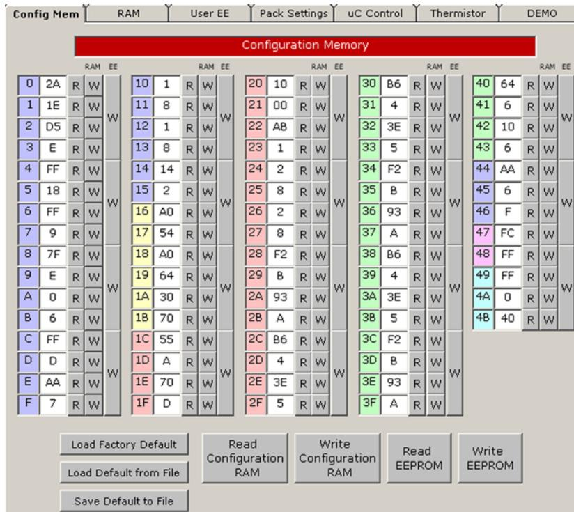
FIGURE 27. ISL94203 GUI - EEPROM ACCESS TAB
