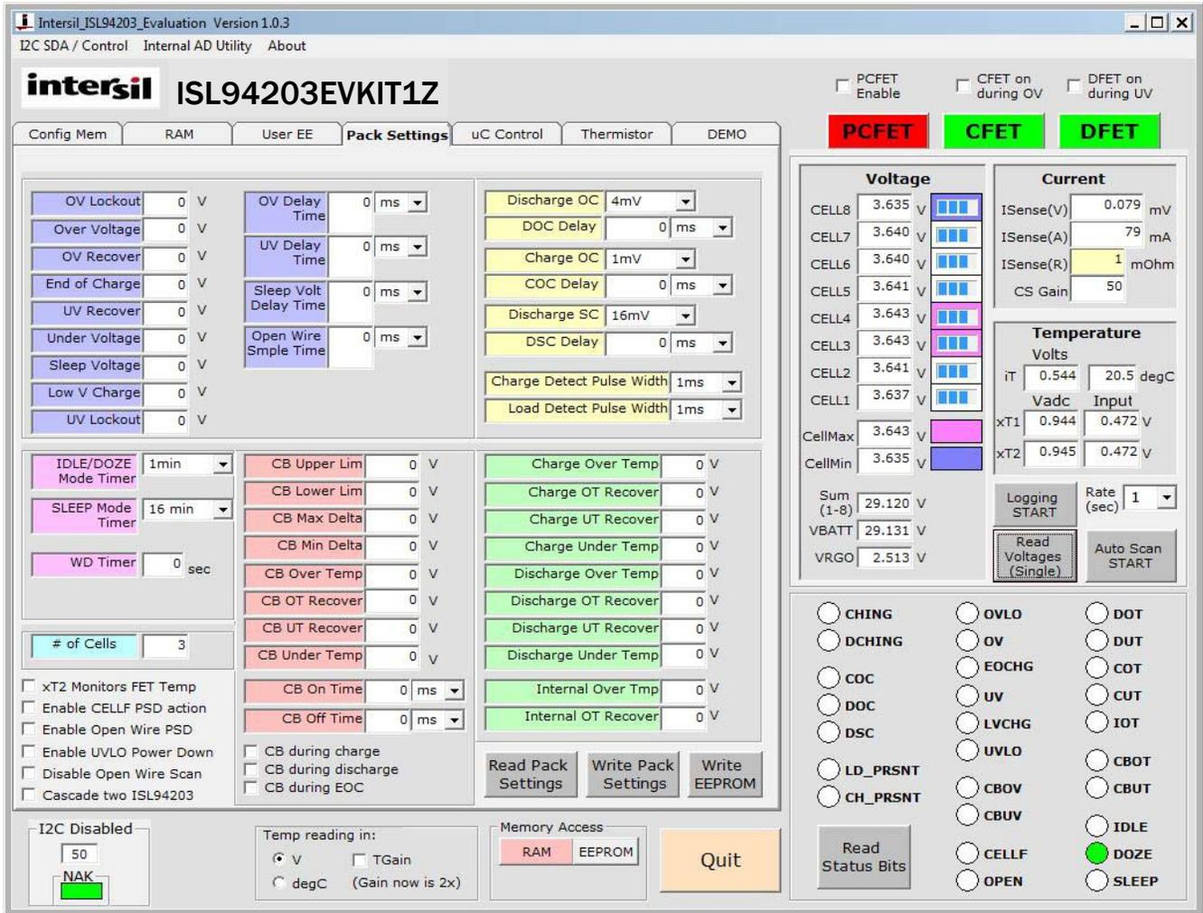
FIGURE 4. MAIN GUI WINDOW SHOWING PACK SETTINGS
