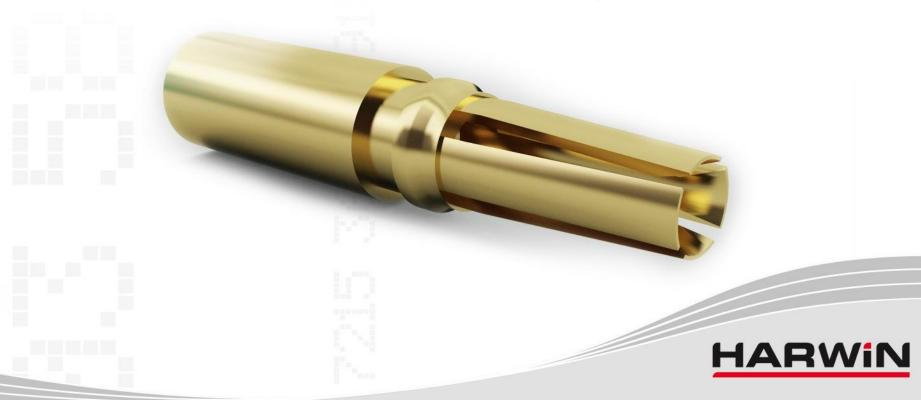
The patented single piece 4-fingered Beryllium Copper female contact gives high electrical performance and sustained mechanical durability. The crimp barrel meets IPC-A-620 specifications. It tolerates extremes of temperature, and withstands high vibration and shock. These contacts are precision-turned on state-of-the-art equipment at the UK headquarters, and plated with a gold finish to resist multiple insertions.
