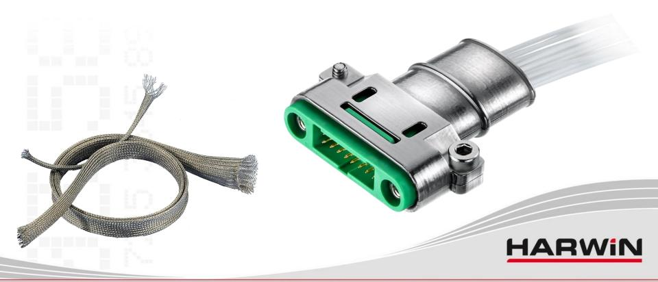
The strong and lightweight machined aluminium backshells provide additional strain relief. They are designed to accommodate flexible, abrasion resistant, metal braiding and are supplied with tie-bands to attach such braiding to the shell. The backshells, together with the braiding, provide shielding for enhanced electrical continuity and effective EMI/RFI protection.
