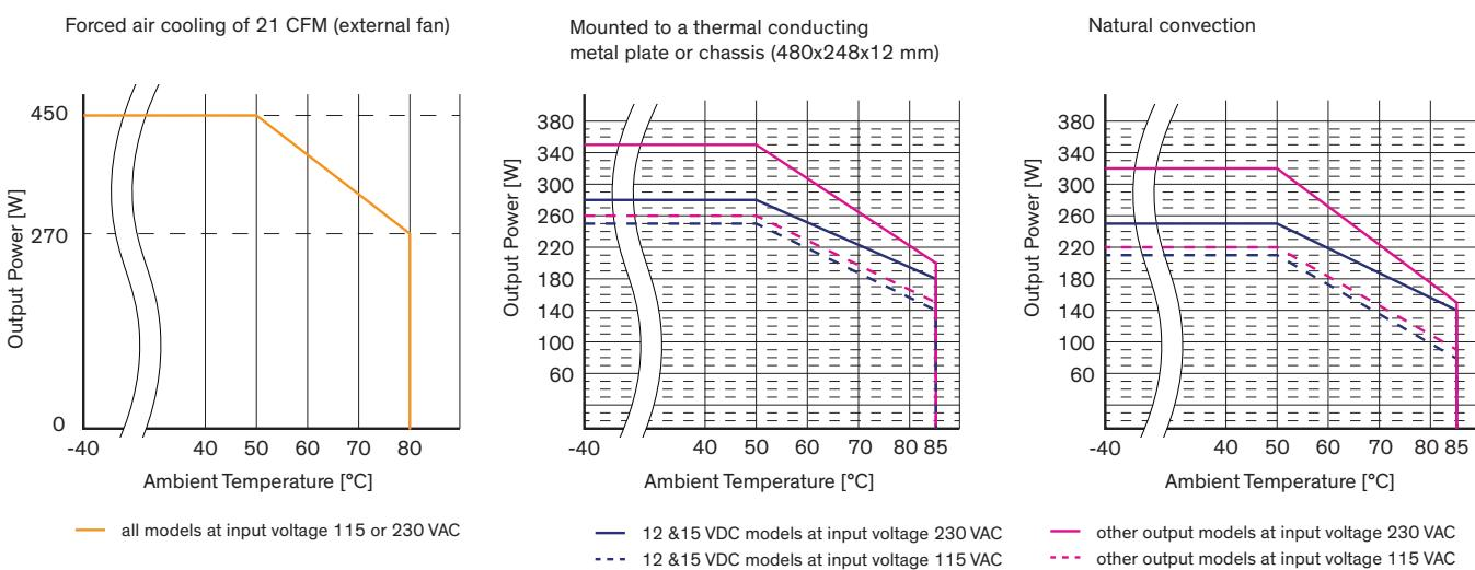
The units are optionally available with casing and internal fan to meet the considerations for forced air cooling (see TPP 450 Series).
