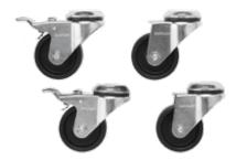
A set of four casters (two locking, two non-locking) that mount directly to the bottom of a ProLine frame, 0-mm or 100-mm Solid Base or a Console. (**Do not use on plinth bases.**) Casters elevate the enclosure 110 mm (4.33) when installed. Caster frames are plated steel with ball-bearing pivots. Caster wheels are made of a black polyamide material. Kit includes M12 mounting hardware. Order separately.
