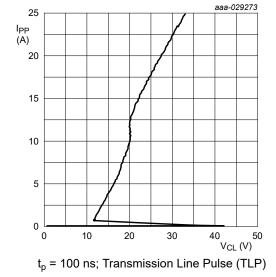
Fig. 5. Positive clamping voltage (TLP); typical values
