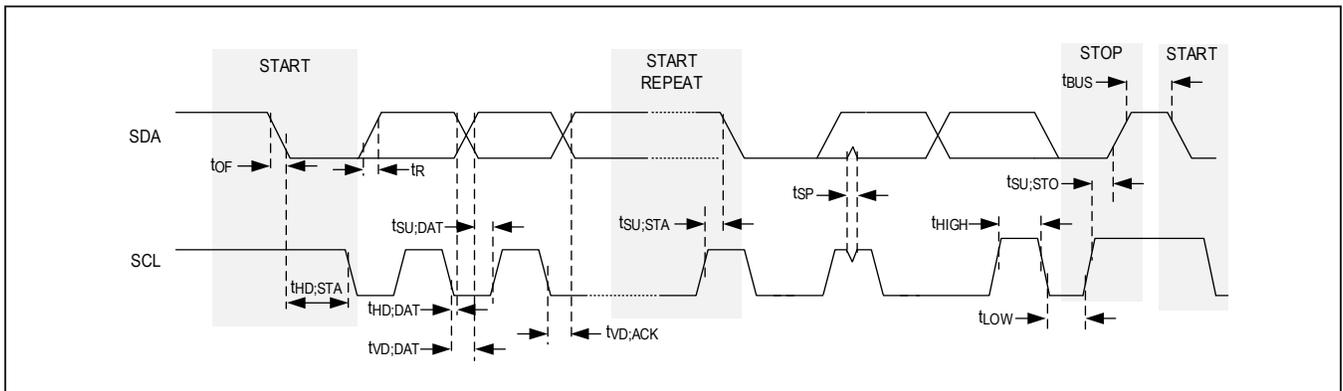
Figure 3. I<sup>2</sup>C Timing Diagram
