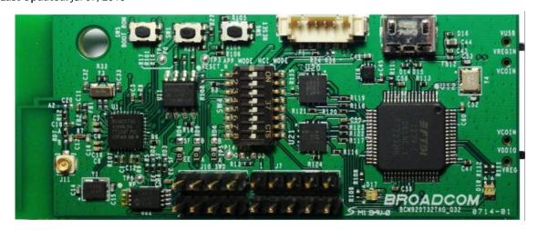
The Cypress WICED™ Smart BCM92073X\_LE\_Kit ("Tag3") is an evaluation board that exposes various pins on the BCM2073X BLE SoC device family for debug, evaluation, and troubleshooting. The BCM2703X BLE SoC family offers Bluetooth Low Energy (BLE)-compliant, stand-alone baseband processors with integrated 2.4 GHz transceivers.
