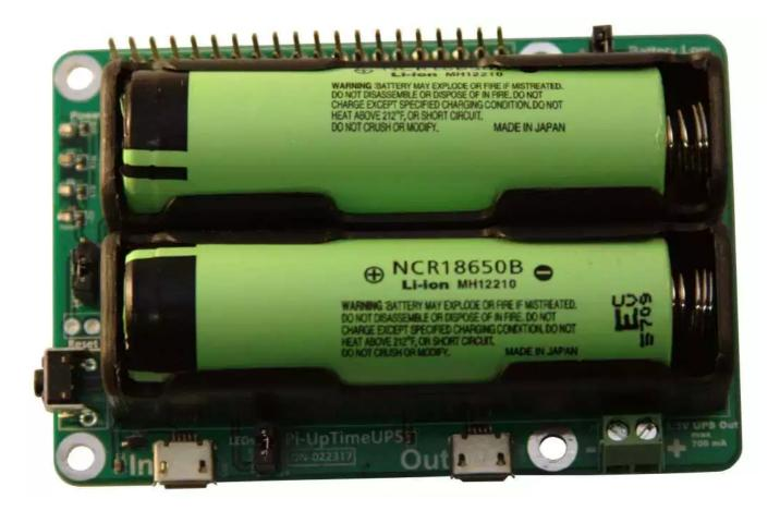
Pi-UpTimeUPS provides power mobility to the Raspberry Pi. Note - batteries or the Raspberry Pi shown are not included.
