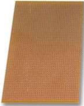
Drilled at 2,54 mm pitch.
