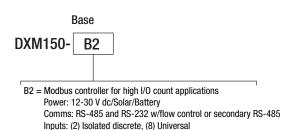
Outputs: (8) PNP/NPN Selectable, (2) Analog Power Out: (2) Courtesy power out; (2) jumper selectable between 2.7 V or battery, 4.2 V or incoming power Radio Configuration
