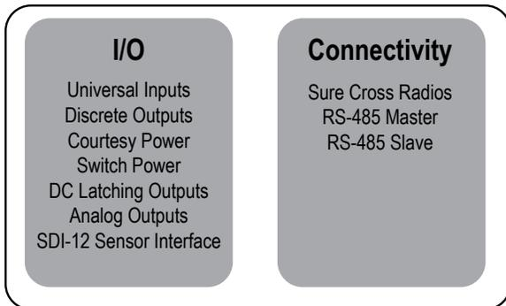
**Inputs/Outputs**—On-board universal and programmable I/O ports connect to local sensors, indicators, and control equipment.
